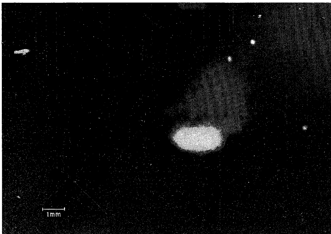
Fig. 3. - Cross-section of the circulating beam.
